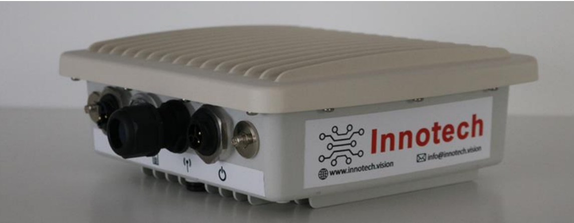
Figure 2: The data processing and communication unit of the WD system before deployment (Banhazi et al. 2024)
